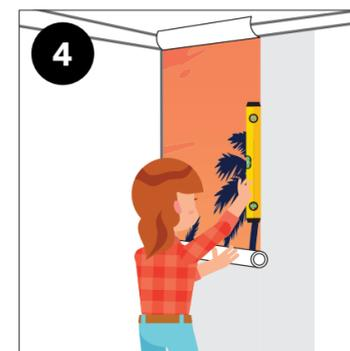
Apply glue to the wall with a roller and apply the first strip to the wall. Start from the top left and make sure that the first strip is straight, using a spirit level or a pencil attached to a piece of string. Is it nice and straight? Make sure to align the next strip carefully!
